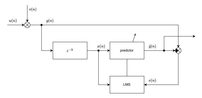
Figure 3: Block diagram of the ALE structure
