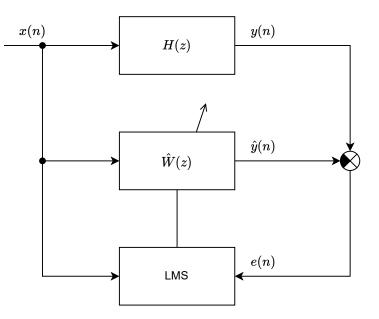
Figure 1: Block diagram of the LMS algorithm
