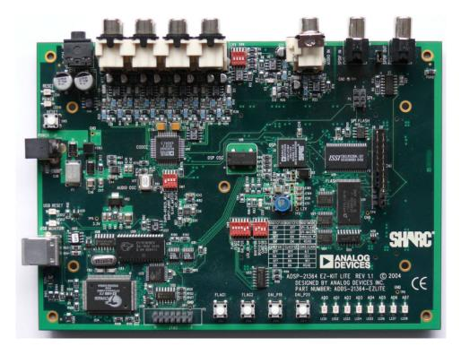
Figure 8: Image of the ADSP-21364 signal processing board
