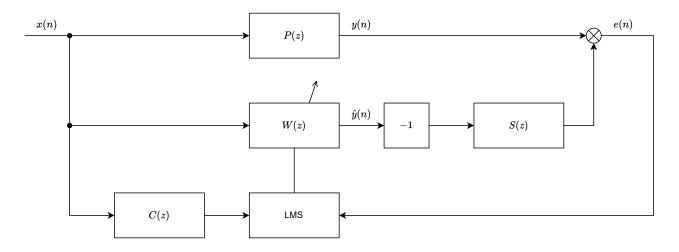
Figure 2: Block diagram of the FxLMS algorithm
