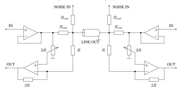
Figure 7: The electronic hybrid circuit to be measured
