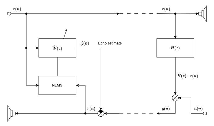
Figure 4: Block diagram of the adaptive echo cancellation structure
