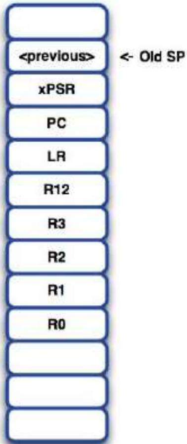
The NVIC will respond to an interrupt with a latency of just six cycles. This includes a microcoded routine to automatically push a set of registers onto the stack.
